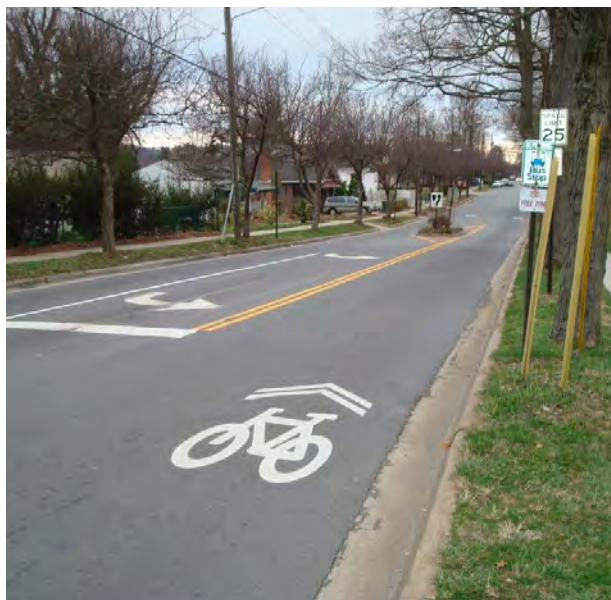
Figure 2.5 Shared lane marking on a suburban roadway. Source: CMAP
